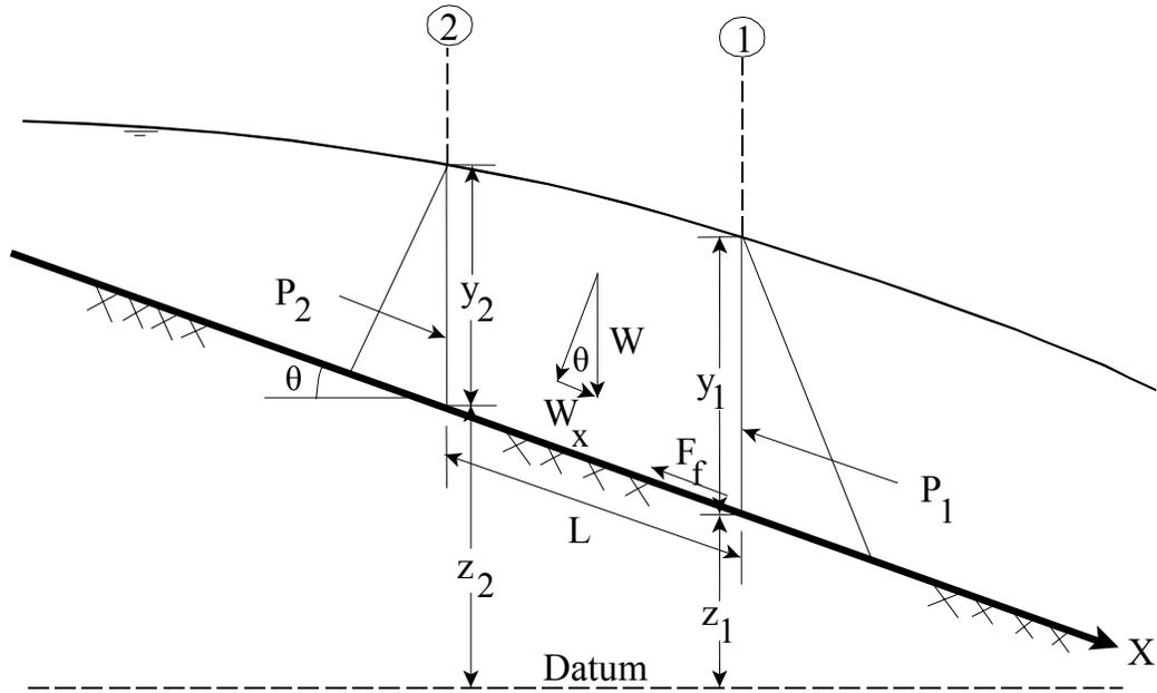
**Figure 2.7 Application of the Momentum Principle**
