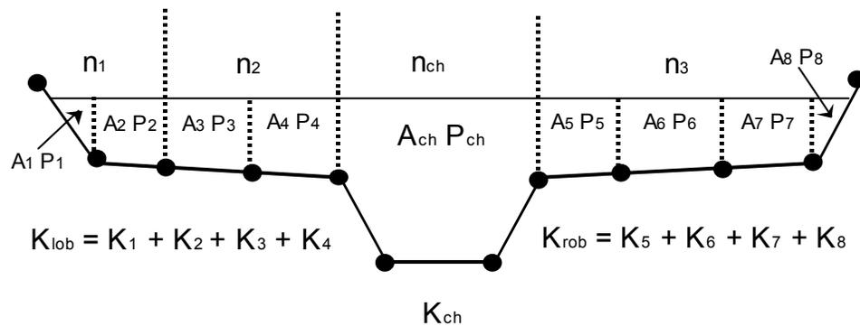
**Figure 2.3 Alternative Conveyance Subdivision Method (HEC-2 style)**
