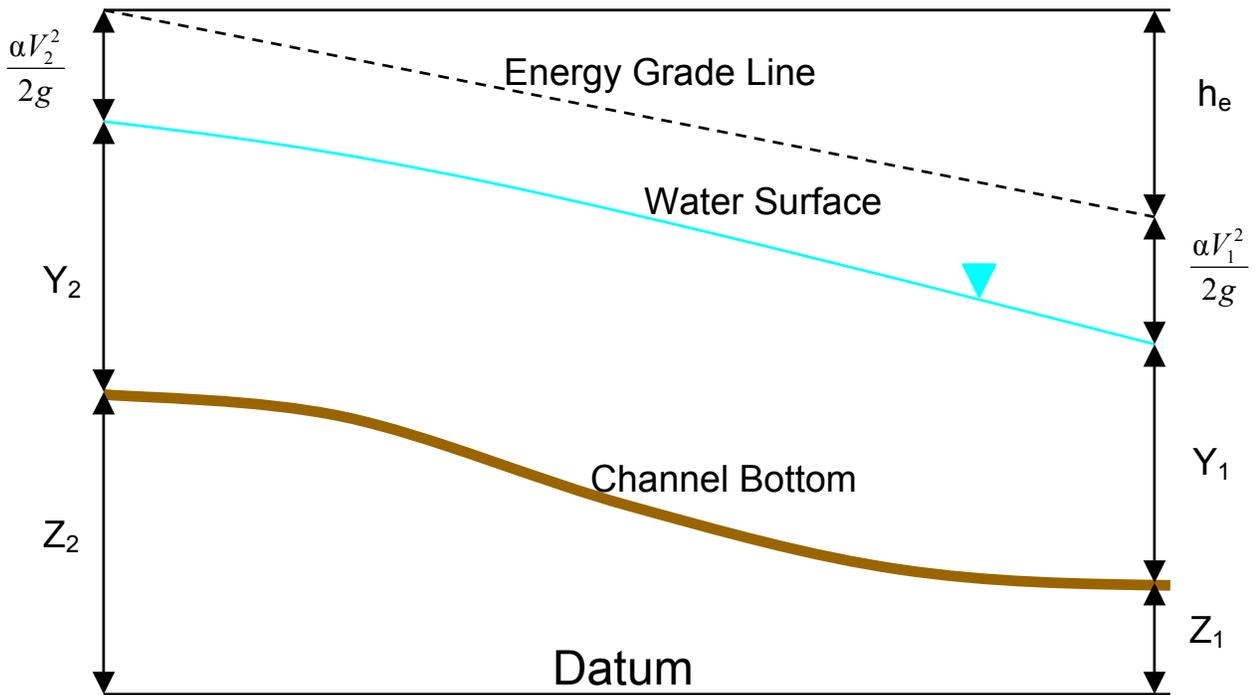
**Figure 2.1 Representation of Terms in the Energy Equation**
